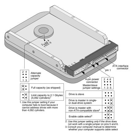
Figure 3. Alternate capacity jumper (ST34340A and ST33230A only) and master/slave jumpers
